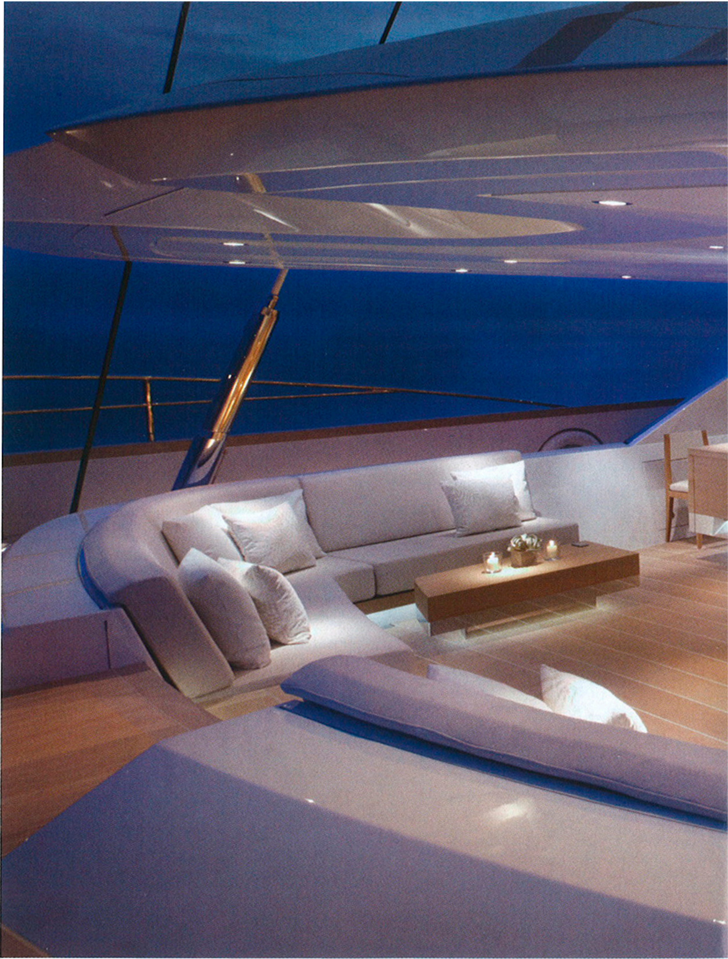
Left: the sunken aft cockpit replaces the need for deckchairs on the aft deck which would roll around when Twizzle is heeled over, and above, the main cockpit
